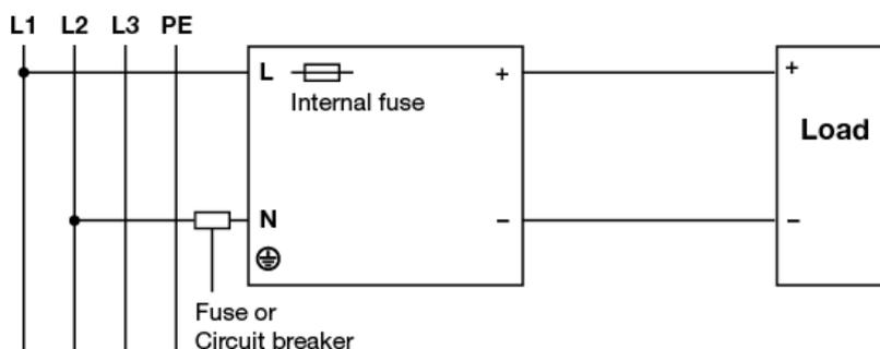
Fig. 4 2 of 3 Phase System Input Operation Connection Diagram
